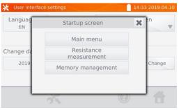
Select the desired startup screen. The screen will be automatically shown after turning the meter on.
