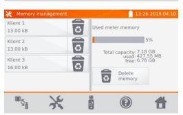
Except reading the % of the used memory, this option allows to clear it. After pressing **Delete memory** all clients are deleted with their objects and measurement results.
